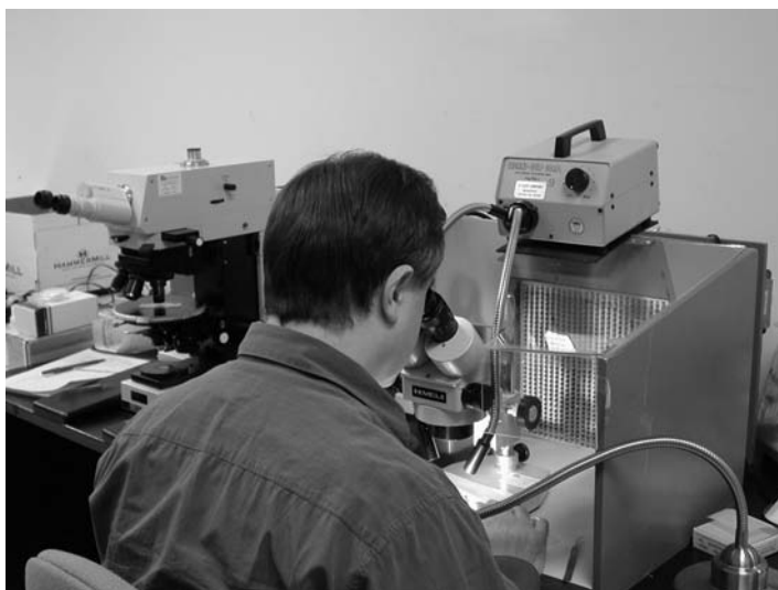
Figure 2.2 Analyst using a stereo-binocular microscope in a HEPA-filtered Hood to examine a bulk sample for asbestos.
