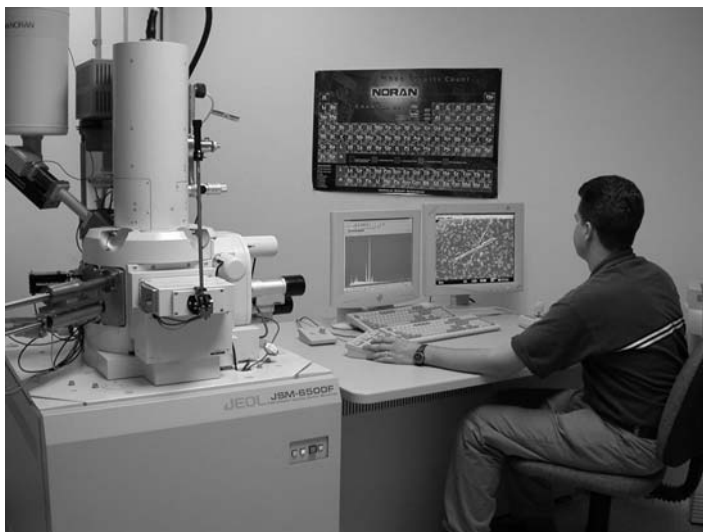
Figure 2.9 Analyst using an SEM for asbestos analysis.
