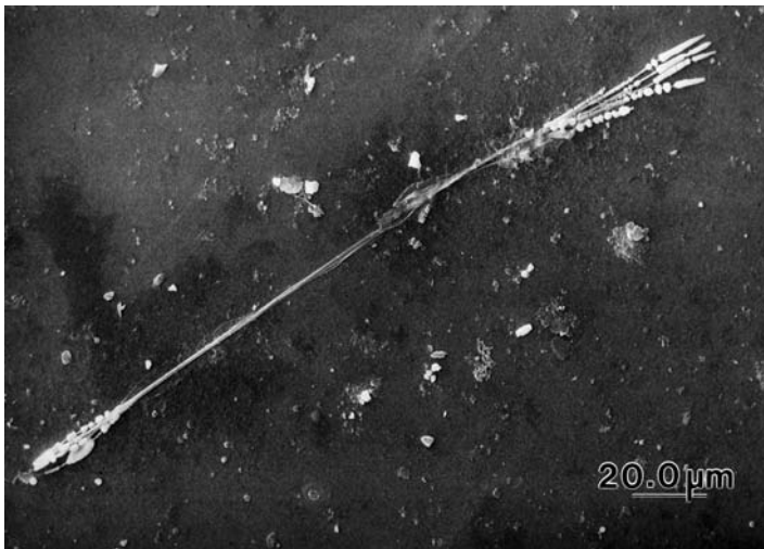
Figure 3.21 Although chrysotile cored ferruginous bodies are less common than those formed on amphibole cores, when longer fibers of chrysotile are inhaled the formation on such cores can occur as indicated in this micrograph. The beaded material representing the ferruginous coating is primarily located on the frayed ends of the fibers.
