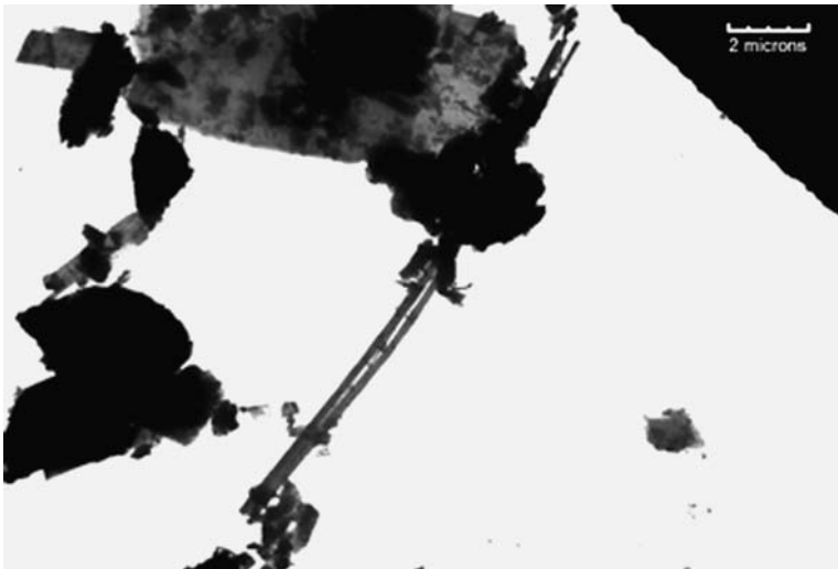
Figure 2.12 TEM image of a tremolite fiber found in a talc sample.
